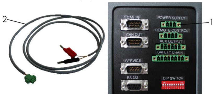
Fig. 4-13 Connect external power supply
