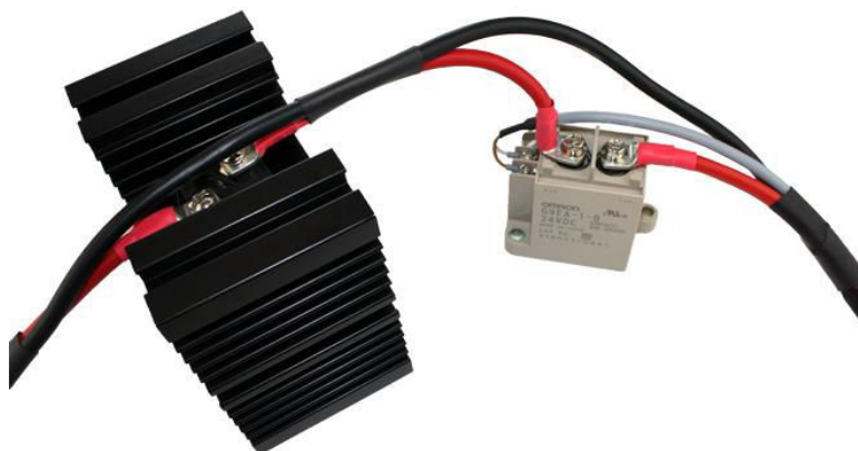
Fig. 3-6 Heat sink with mounted reverse current diode and connected load relay
