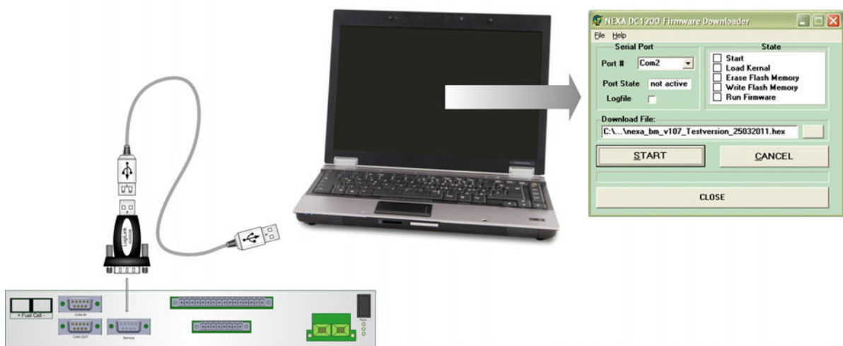
Abb. 1-1 Establish communication between Nexa® DC1200 and the PC
