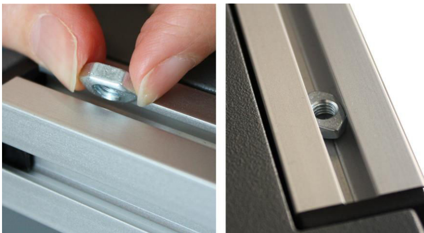
Fig. 10-1 Insert sliding block in profile
