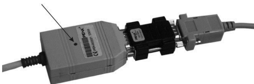
Fig. 5-3 Status display at CAN-USB converter
