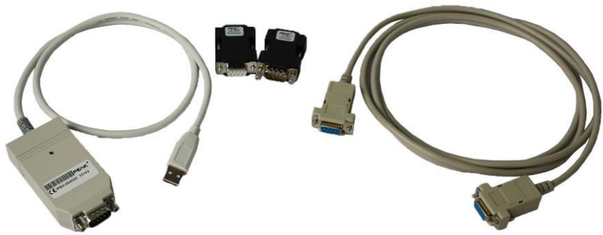
Fig. 3-7 CAN-USB converter, 2 terminating resistors and CAN cable
