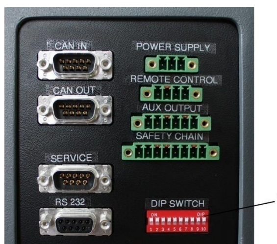
Fig. 10-2 DIP switches on connection panel
