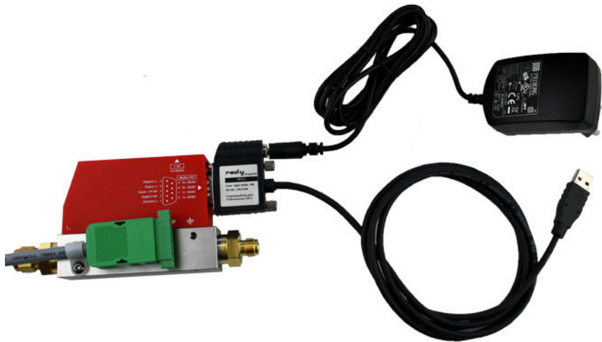
Fig. 4-2 Connect data interface to PC
