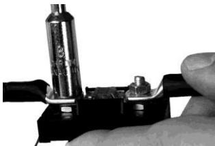
Mounting the fuse
