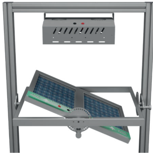
Figure-36. Photovoltaic Panel Depending on the Sun's In-Day Movement, the panels are moved along this axis
