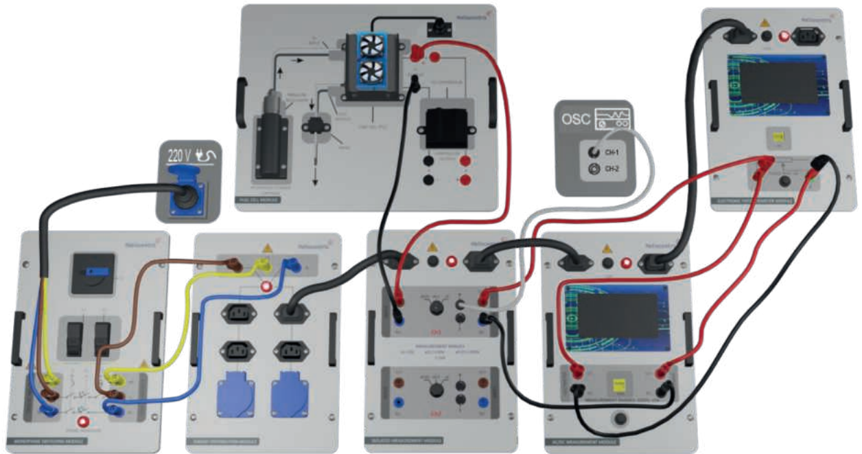
Figure-82. Installation Image of Examination of Hydrogen Fuel Cell Output Voltage Under Load with Oscilloscope
