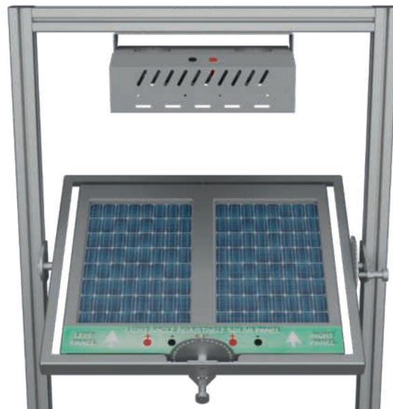
Figure-40. Due to the Season Change of the Photovoltaic Panel, the panels are moved along this axis.
